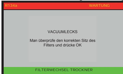
Check filter tightening and press OK to restart the vacuum check.
