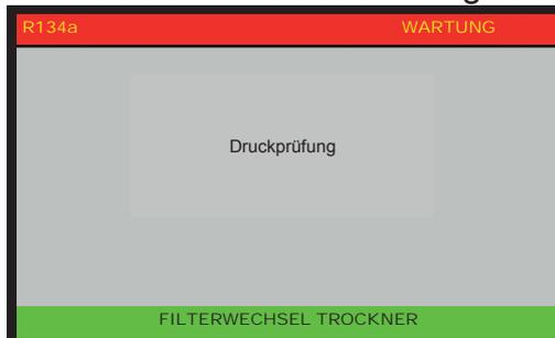
17) If leaks are detected the following screen will be displayed:
